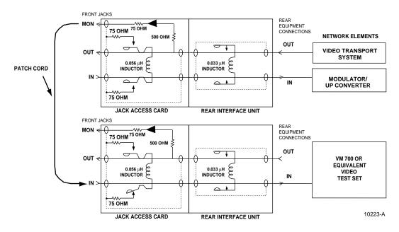
Figure 28. Non-Intrusive Test of Transport Feed
